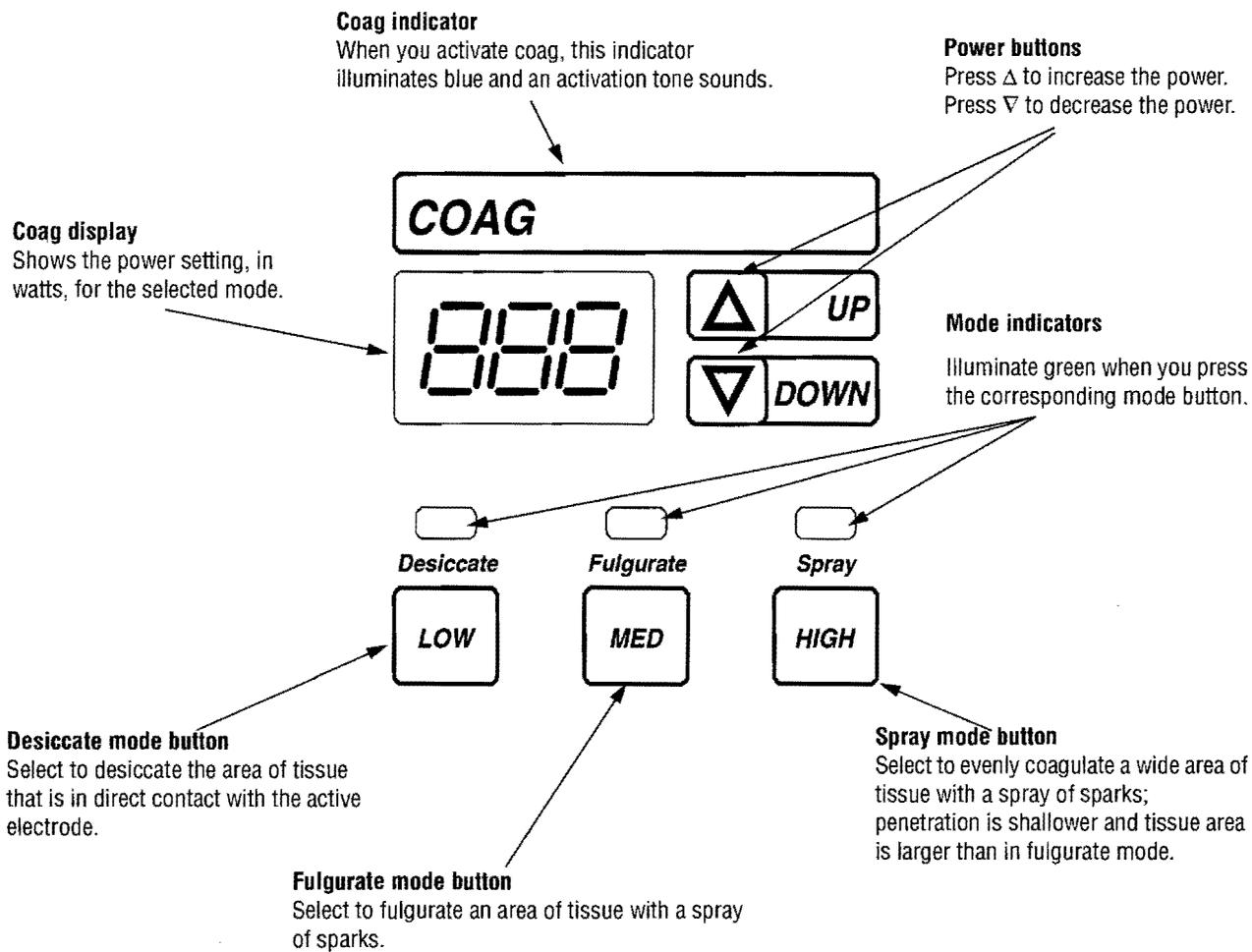
This unit is equipped with an additional fulgurate mode which incorporates a lower crest factor (LCF) than the factory default fulgurate mode. Details about this additional fulgurate mode, LCF fulgurate, are provided later in this manual.
