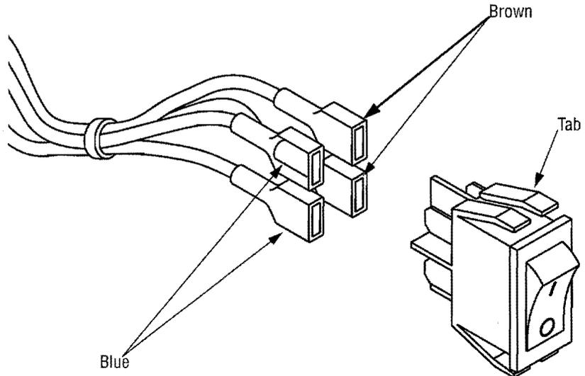
3. Remove the heat shrink from the cables and old switch.
