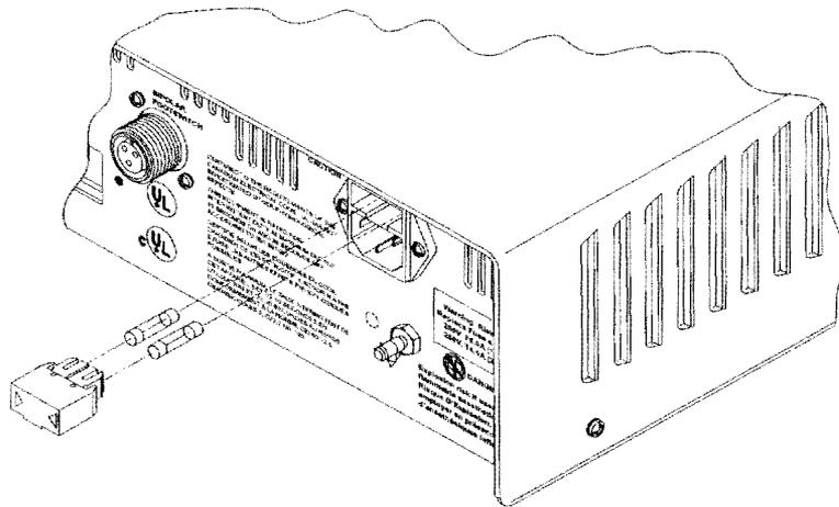
3. Use a fuse puller to remove each blown fuse from the fuse drawer.
