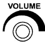
Turn to adjust the volume of the tones that sound when the generator is activated (activation tone). To ensure that the surgical team is alerted to inadvertent activation, these tones cannot be silenced.
